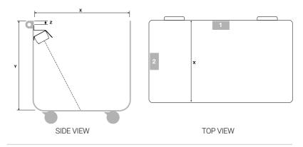
**Fill Height** is the measurement from the bottom of the container to where you establish 100% fullness (see **Red Line** below). The **Fill Gap** is the measurement from the sensor to the 100% fullness level. (see **Green Line** below).
